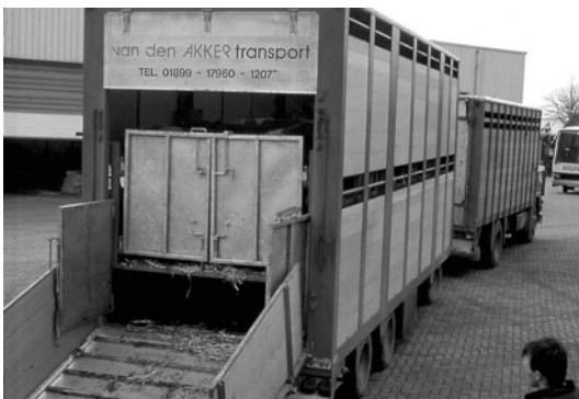
Fig. 21.1. Vehicle with hydraulic floor lift (photograph courtesy of D.M. Broom).
