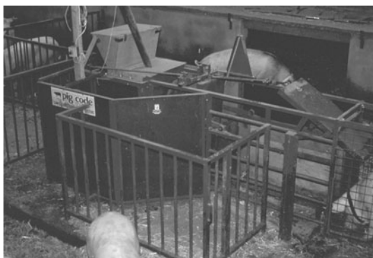
Fig. 29.2. Sows kept in groups have access to this electronic sow-feeder that delivers food to them, after their entry, only if they have not received their ration for the day. The sow should have a front exit to the feeder (photograph courtesy of D.M. Broom).
